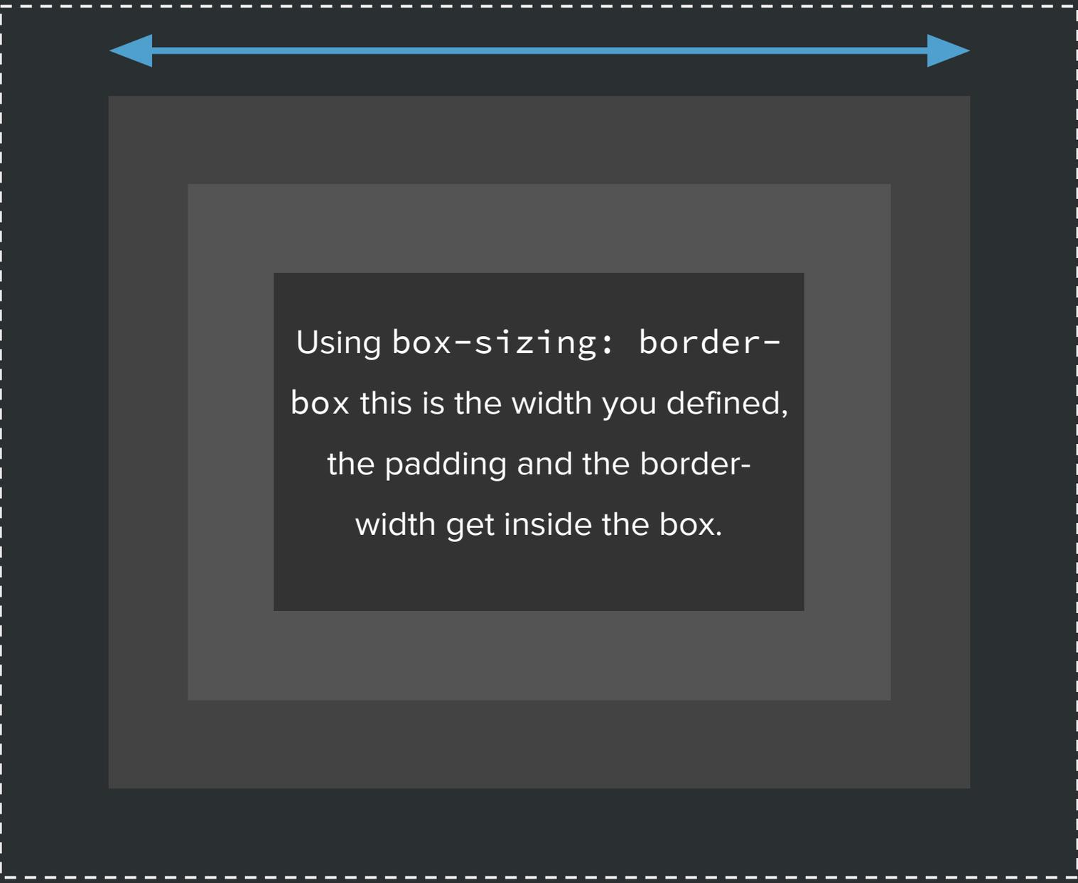
The diagram consists of three nested rectangles. The outermost rectangle is defined by a dashed white border. Inside it is a medium-gray rectangle, and inside that is a dark-gray rectangle. A blue double-headed arrow is positioned at the top, spanning the width of the dashed white border. The text is centered within the dark-gray rectangle.
